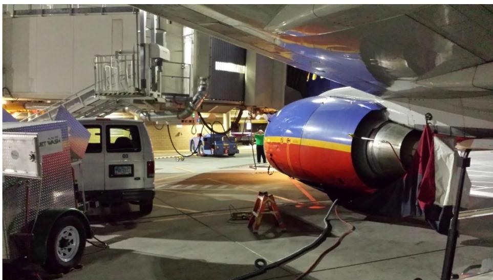
The AJW Wash System consists of three tanks: Two 100 Gallon tanks hold pure heated de-ionized water (detergent or alcohol is available if needed) and one 55 Gallon tank holds waste water collected by the Effluent Collection Suit.
